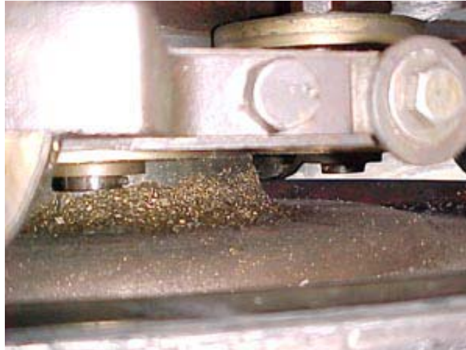
Figure 3-4. Evidence of Metal Shavings.
