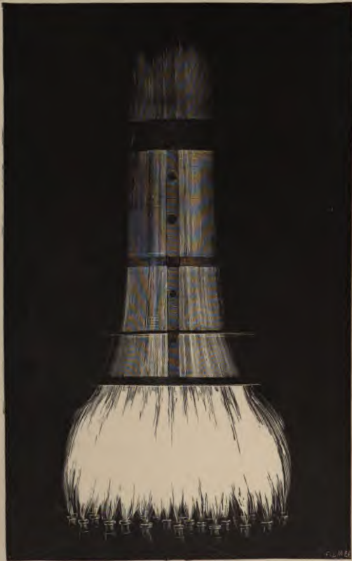
THE IRISH GAS LIGHT FOR LIGHT-HOUSES—108 Jets.
