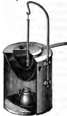
Apparatus for testing the flashing-point.
