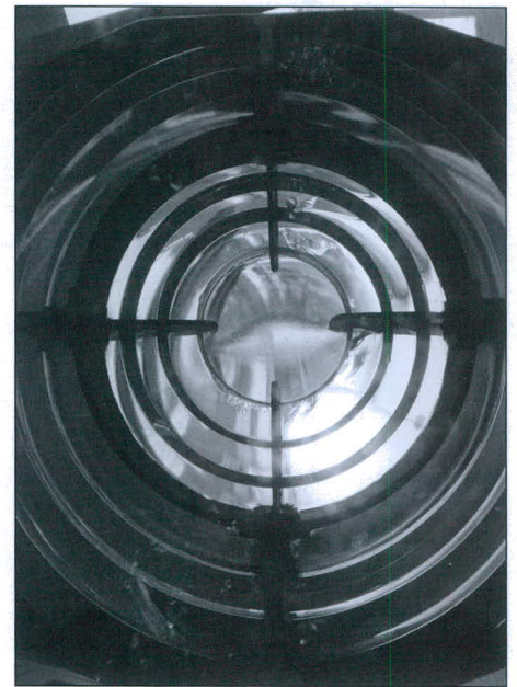
A unique double lens illuminated the Neuer Leuchtturm when it was first commissioned. The lens panels were situated on a revolving table opposite each other. Today the lens is on display at the base of the lighthouse. Author photo.
