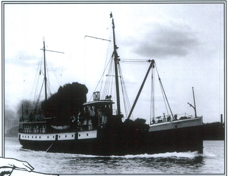
Above - The Lighthouse Service Tender Marigold under full steam. This 160 foot long tender was constructed in 1890. The boxy device on the roof of the pilot house is a radiobeacon antenna and dates the photo after 1923. Official Coast Guard photo.
