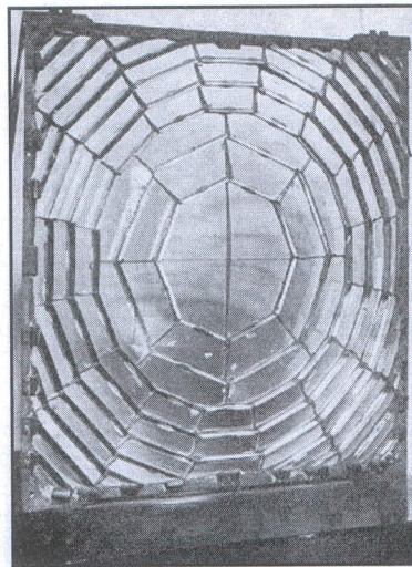
Fresnel's polygonal bulls-eye lens flash panel (early in 1821). Photo from Centenaire D'Augustin Fresnel .
