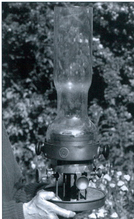
A five-wick lamp used in one of the Cape Ann Light Station towers and still on the island. Photo courtesy of the Thacher Island Association.
